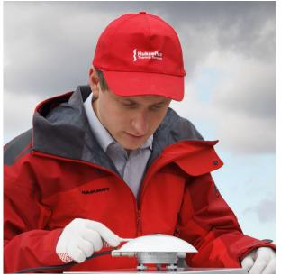
Figure 3 IR20 pyrgeometer being prepared for application.
