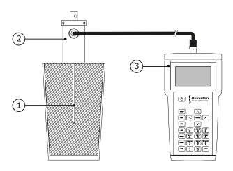
**Figure 1** MTN02 system in operation: thermal needle TP07 (1), mounted on the insertion tool IT03 (2), is inserted into the soil sample. The user performs control and readout of the experiment from the CRU02 (3), using its keyboard and LCD.
