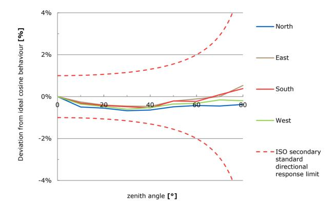
**Figure 2.3** *Directional response of a SR20-D2 pyranometer of 4 azimuth angles, compared to spectrally flat Class A (secondary standard) limits.*
