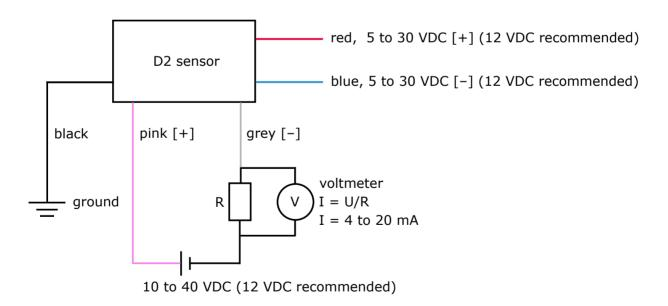
**Figure 5.5.2** Electrical diagram of the connection of SR20-D2 to a typical voltmeter or data logger with the capacity to measure voltage signals. Usually a 100  $\Omega$  shunt resistor (R) is used to convert the current to a voltage. SR20-D2 operates on a supply voltage of 5 to 30 VDC. In addition, 10 to 40 VDC is needed for the 4 -20 mA function.
