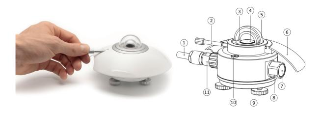
Figure 5.2.1 Installation and removal of SR20-D2's sun screen.
