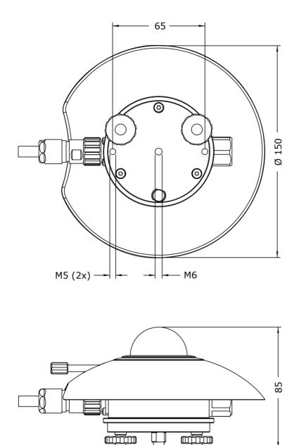
**Figure 3.2.1** *Dimensions of SR20-D2 in x 10<sup>-3</sup> m.*
