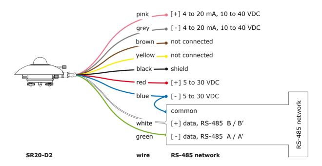
Figure 6.4.1 Connecting SR20-D2 to a typical RS-485 network.
