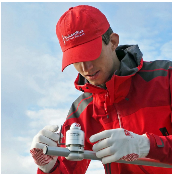
Figure 2 Easy levelling of SR05 on its tube mount with ball levelling
