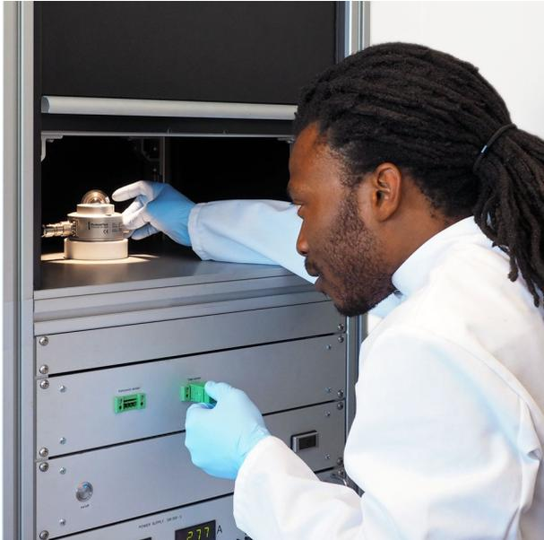
**Figure 3** at work with a typical calibration system at Hukseflux, in this case calibrating an ISO secondary standard pyranometer
