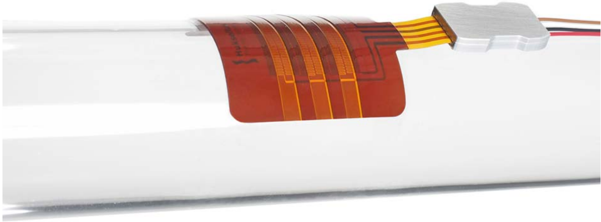
Figure 2.2 Heat flux from the back side to the front side (side with sticker, logo readable) generates a positive voltage output signal
