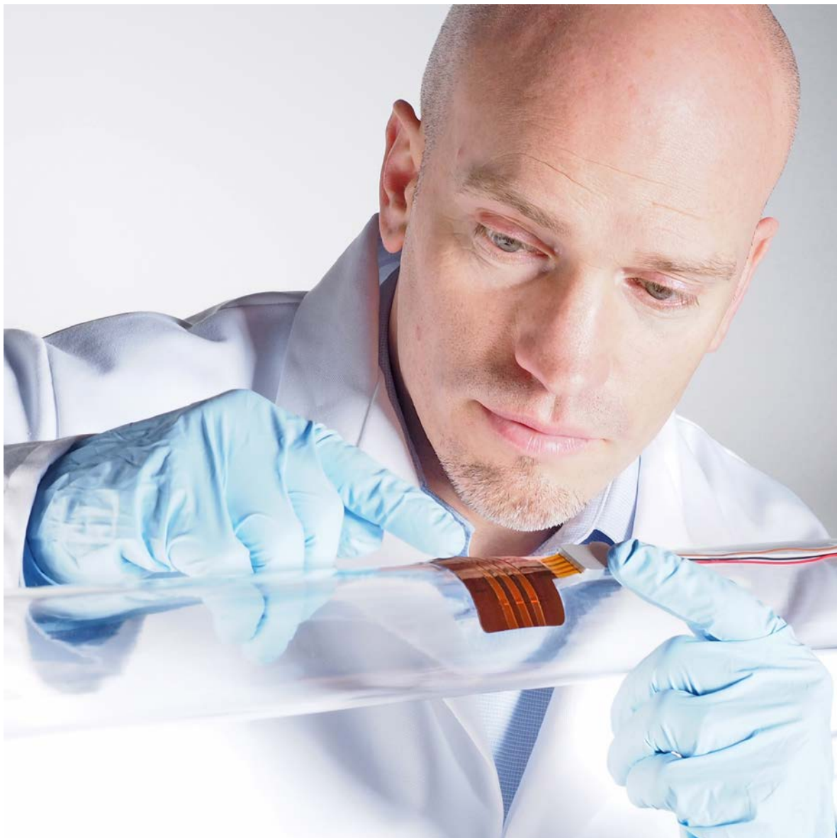
Figure 4.1.1 Example of a flexible foil heat flux sensor being installed on a pipe. The sensor is mounted on a well prepared flat surface. Wiring must be provided with strain relief.
