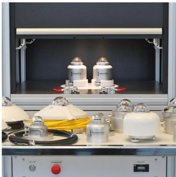
Figure 1 Calibration of all major pyranometer brands.
