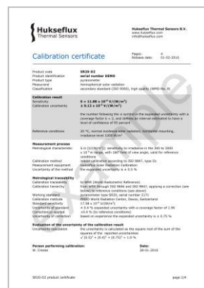
Figure 2 A calibration certificate is supplied with each sensor documenting traceability and uncertainty evaluation.
