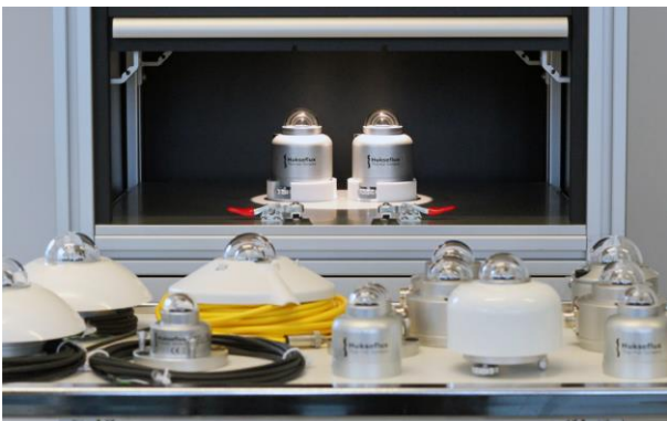
Figure 1 calibration of all major pyranometer brands
