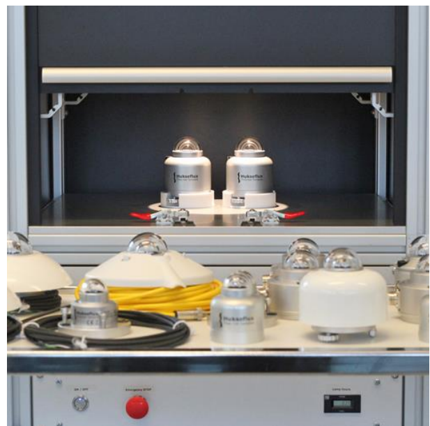
Figure 2 calibration of all major pyranometer brands
