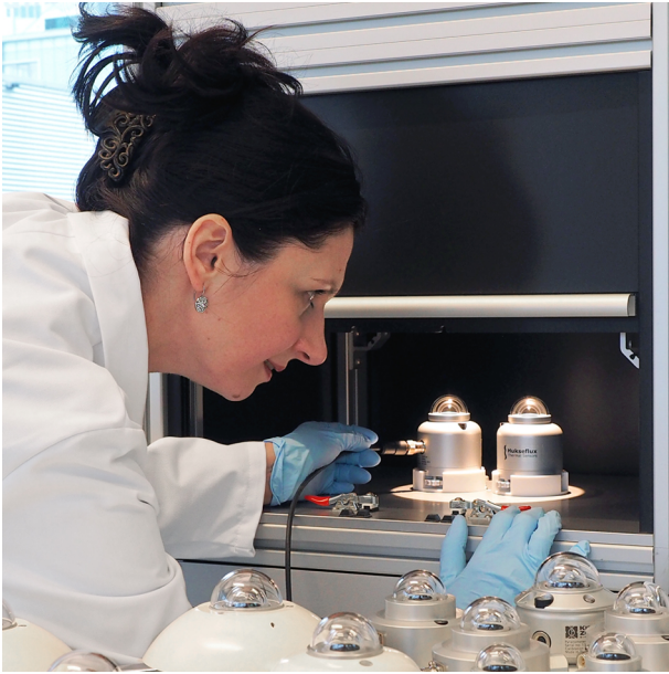
Figure 3 a typical calibration system at Hukseflux
