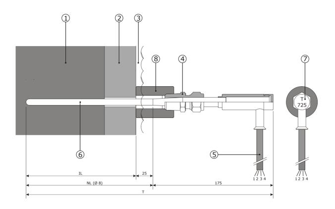
**Figure 3.2.1** *NF01 standard version for operation in the furnace lining (graphite or brick) part of the furnace wall: (2) steel shell, (3) water, (1) graphite, (8) shell coupling, (4) screwed coupling, (5) cable, (6) needle type heat flux and temperature sensor.*
