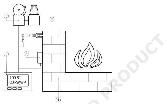
**Figure 0.5** Monitoring of furnaces and ovens: (1) needle type heat flux & temperature sensor NF01, (2) surface heat flux & temperature sensor model HF01 (not discussed in this document), (3) readout unit, (4) brick, (5) alarm/warning system
