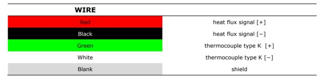
**Table 4.1.2** The electrical connection of NF01. Optional ANSI colour code; the ANSI code for thermocouple K is yellow / red.
