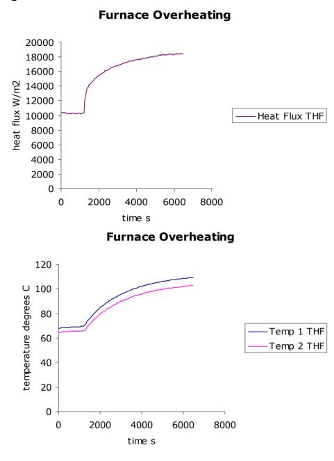
**Figure 7.2.1** *Example 1: simulation of furnace overheating. Normal operation of the furnace until about 1000 s. Form then on the furnace starts overheating. In case of furnace overheating all temperatures as well as the heat flux rise. In this case the heat flux is increased by a factor 1.8.*
