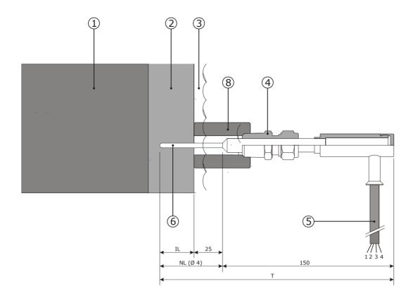
**Figure 3.2.2** *NF01* optional  $4 \times 10^{-3}$  m diameter version for operation in the water cooled part (shell) of the furnace wall: (2) steel shell, (3) water cooled, (1) graphite, (8) shell coupling, (4) screwed coupling, (5) cable, (6) needle type heat flux and temperature sensor.
