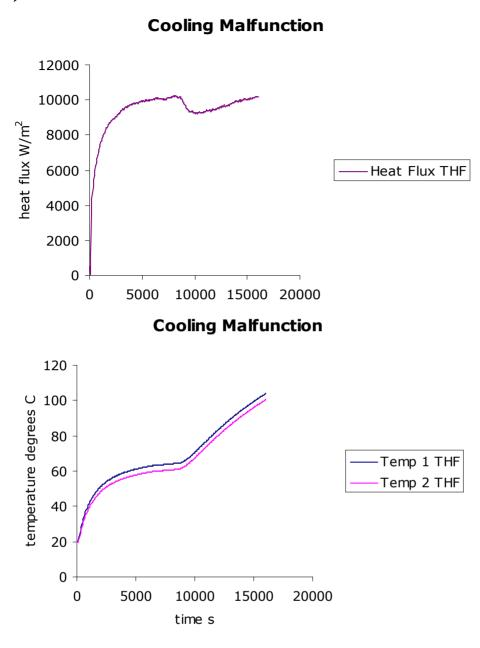
**Figure 7.2.2** *Example 2: simulation of cooling malfunction. Around 8000 s after initial start-up of the furnace, the water cooling is stopped. The temperatures rise quickly but the heat flux, after a temporary dip caused by thermal loading, stays close to normal. It will eventually stabilise close to the original heat flux at a higher absolute temperature. Please note that the heat flux signal has been corrected for the temperature dependence of the thermal conductivity.*
