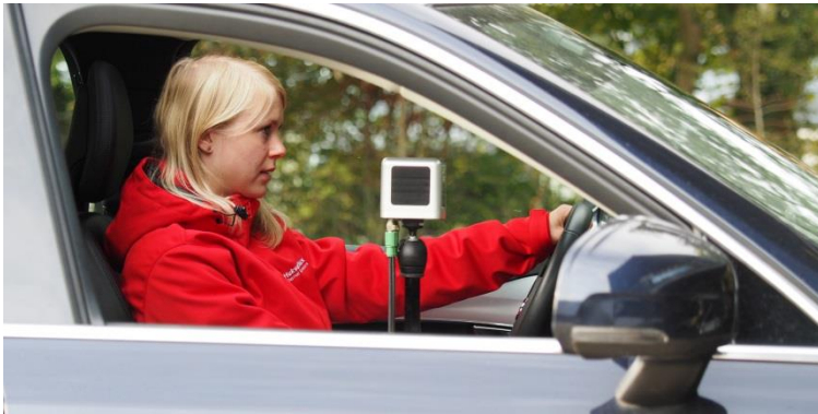
Image 0.2 TCOM01 mannequin applied in car passenger comfort testing
