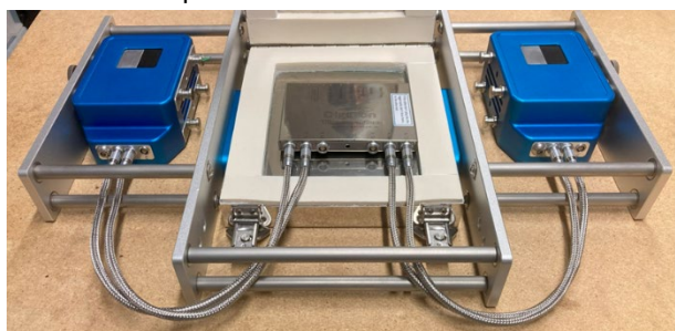
Figure 3 Two 60 mm sensor heads, each equipped with a black and silver coated FHF05 sensor, installed on a frame with a data logger and a thermal barrier.
