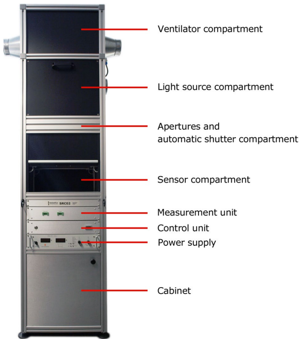
Figure 2 Example of a typical test facility designed by Hukseflux: SRC02. 19-inch rack, height 2.4 m. (see also figure 3).
