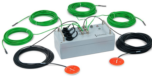
Figure 7 Example of a measuring system designed by Hukseflux engineering. Measuring system for analysis of the thermal resistance and the thermal transmittance of building elements by in-situ measurement. TRSYS02 is used for measurements according to ISO 9869 and ASTM C1155 / C1046 standards.
