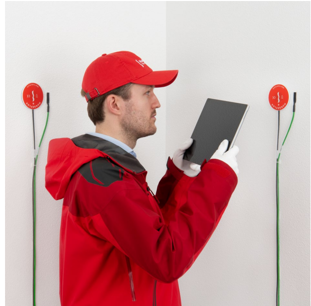
Figure 8 TRSYS02 in use: on-site measurement of the building envelope thermal resistance.
