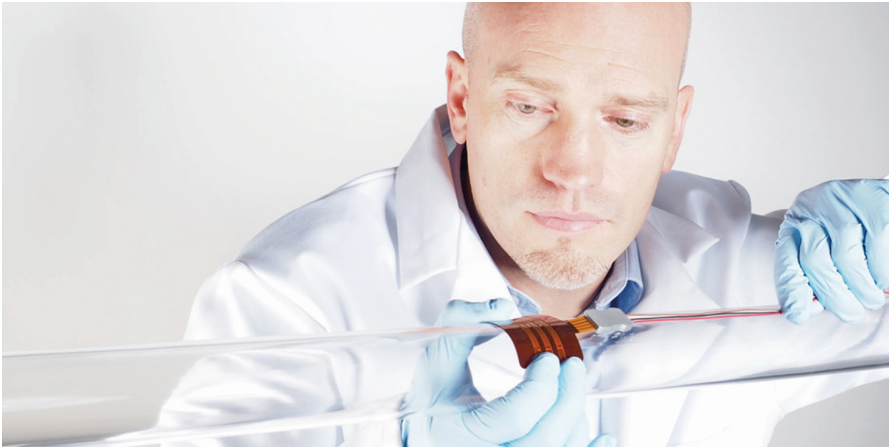
Figure 1 a flexible heat flux sensor on a tube surface measuring heat flux between the tube and its environment.
