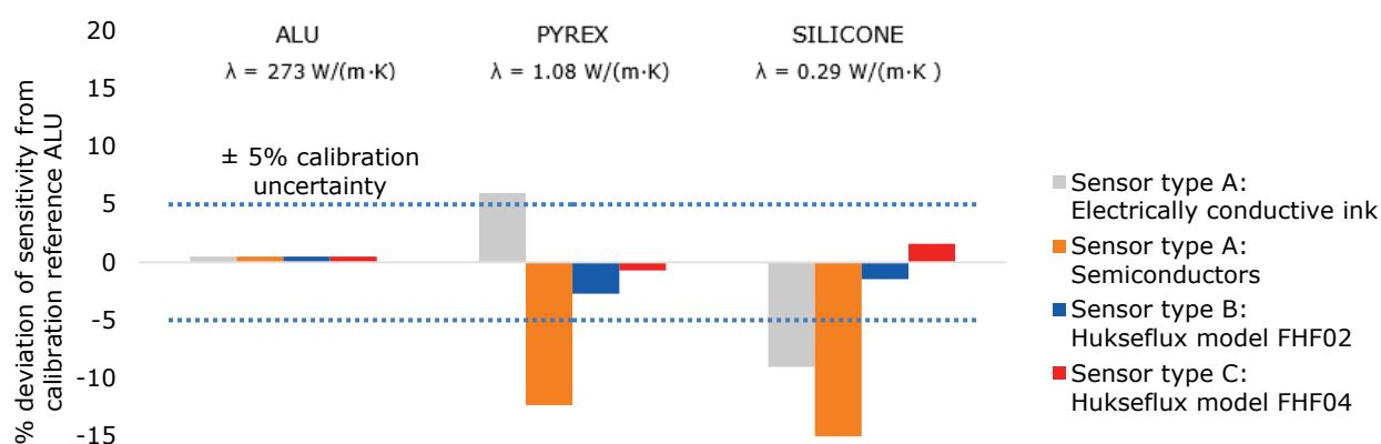
**Figure 6** Thermal conductivity dependence of three sensor types. Two "type A" sensors were tested: one with a thermopile made of electrically conductive inks and the other made of semiconductors. The calibration uncertainty is 5 %. Sensor type A makes up to 15 % error when the thermal conductivity of the environment changes. Errors made with type B and C sensors are negligible.
