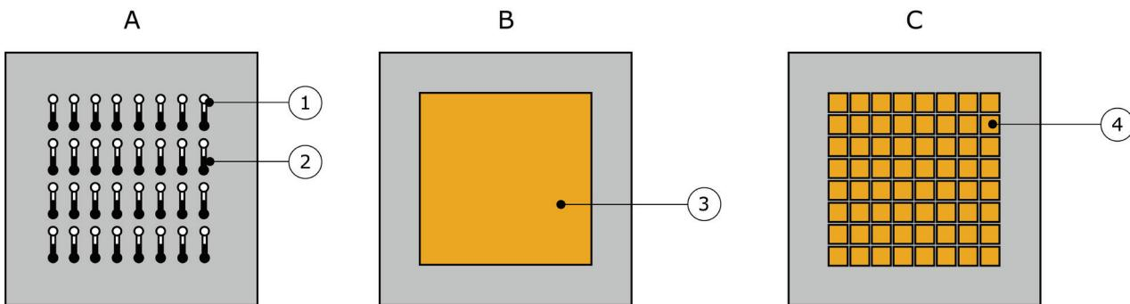
**Figure 5** A: sensor without a spreader. One thermopile alloy (1), other thermopile alloy (2) In B and C, the thermopile is covered by spreaders. B: sensor with a single large spreader (3) C: sensor with multiple small spreaders (4)
