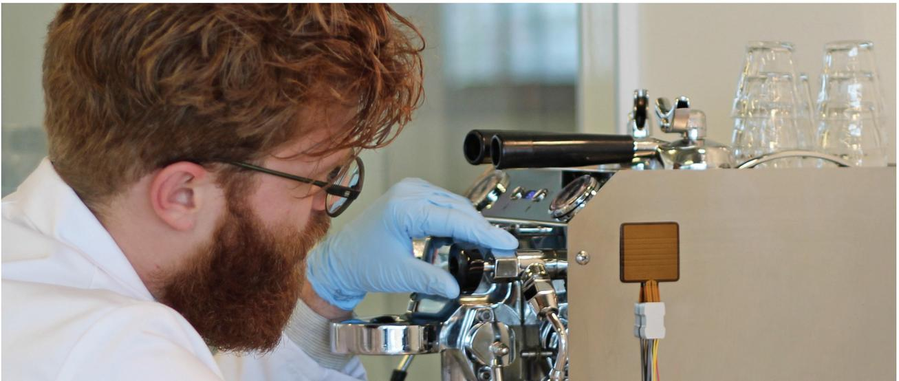
**Figure 1** heat flux sensor on a metal surface to study heat losses of an espresso machine
