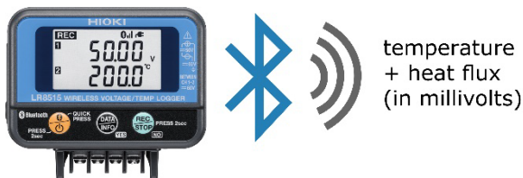
Figure 2 Hioki LR8515 can transmit measurements of 1 sensor via Bluetooth
