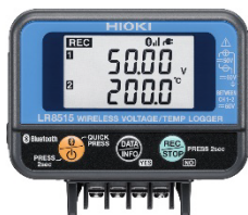
Figure 2 Hioki LR8515 can transmit measurements of 1 sensor via Bluetooth.
