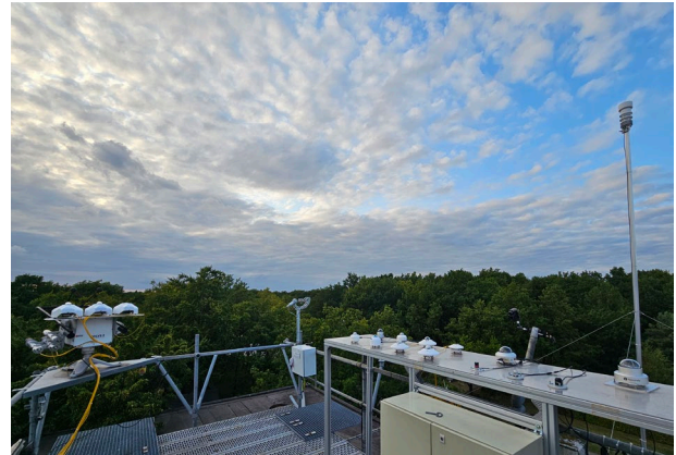
Figure 5 Rooftop setup at Denmark Technical University showing a collection of pyranometers, diffusometers, and a rotating shadowband pyranometer. Source: DTU, Adam Jensen.
