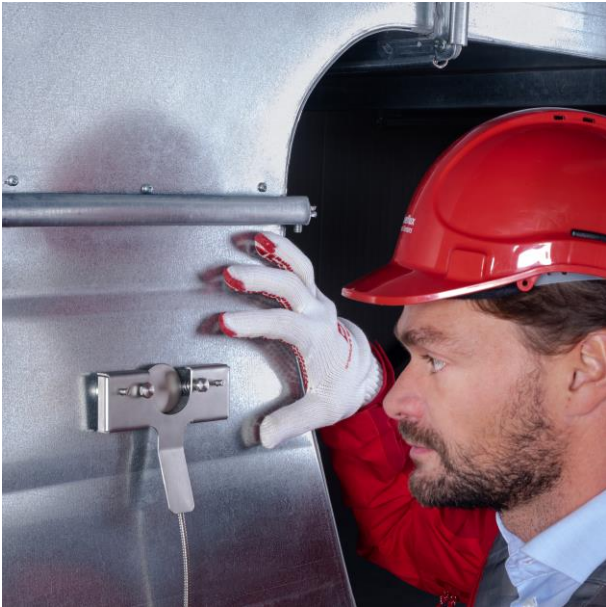
Figure 3 verification of thermal behaviour of industrial equipment with the very robust IHF02 sensor
