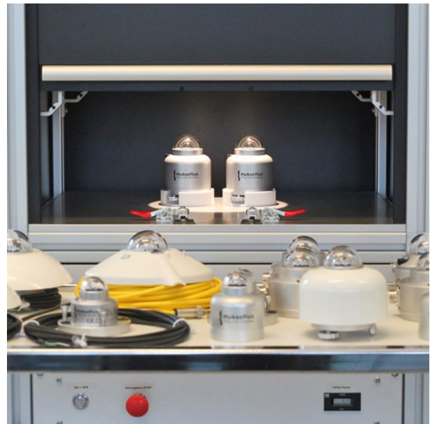
Figure 2 calibration of all major pyranometer brands
