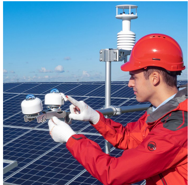
Figure 3 two SR30 secondary standard pyranometers with digital output for GHI (global horizontal irradiance) and POA (plane of array) measurement applications
