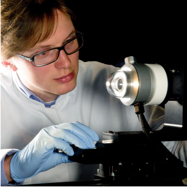
Figure 6 Individual testing of every instrument; Hukseflux performs individual testing of temperature response and directional response of all secondary standard instruments
