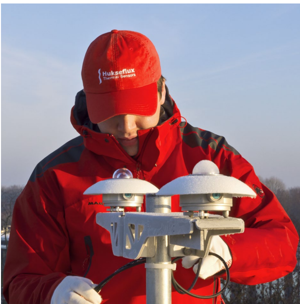
Figure 1 Improving data availability and measurement uncertainty; heated versus unheated instruments
