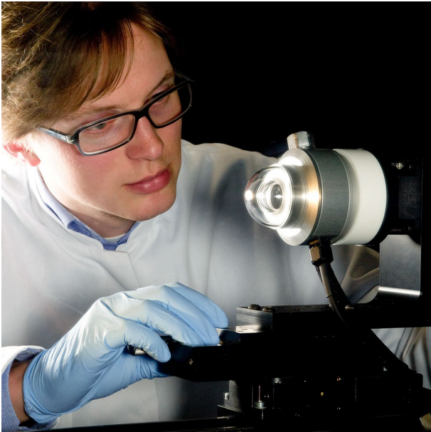
Figure 6 Individual testing of every instrument; Hukseflux performs individual testing of temperature response and directional response of all Class A instruments.
