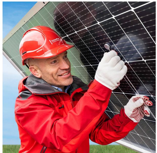
Figure 7 PVMT01 installed on the rear side of a PV module. The sensors are preferably installed at the centre of a cell close to the centre of the module. IEC requires 3 sensors per monitoring station.
