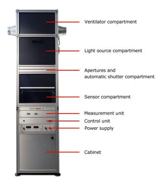
Figure 1 SRC02 indoor pyranometer calibration system
