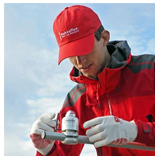
Figure 3 The Class C model SR05 is smaller than the Class A and B pyranometers and has slightly different mounting and levelling. The optional ball levelling and tube mount, TMBL01 (including BL01), allow for easy installation, levelling and removal.
