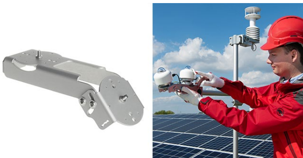
Figure 4 Two SR200-D1 pyranometers on a PMF02 dual pyranometer mounting fixture, one tilted for Plane of Array (POA) measurement, and another mounted horizontally for Global Horizontal Irradiance (GHI) measurement.
