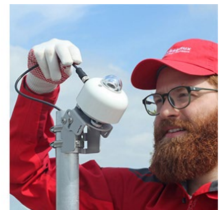
Figure 7 Installation of one AMF02 albedometer mounting kit and two SR20 pyranometers, mounted with one ALF01 levelling fixture on a crossarm with crossarm bracket CMF01.
