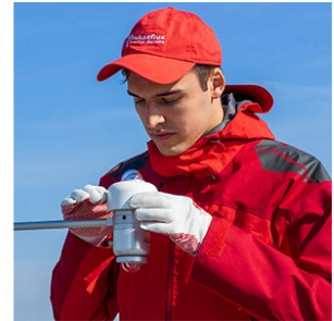
Figure 5 The SRA300-D1 is composed of one AMF03 and two SR300-D1 pyranometers.
