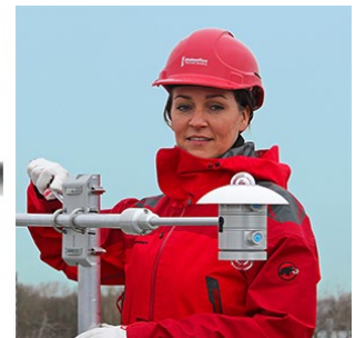
Figure 7 Installation of one AMF02 albedometer mounting kit and two SR20 pyranometers, mounted with one ALF01 levelling fixture on a crossarm with crossarm bracket CMF01.
