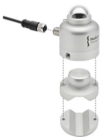
Figure 3 The Class C model SR05 is smaller than the Class A and B pyranometers and has slightly different mounting and levelling. The optional ball levelling and tube mount, TMBL01 (including BL01), allow for easy installation, levelling and removal.
