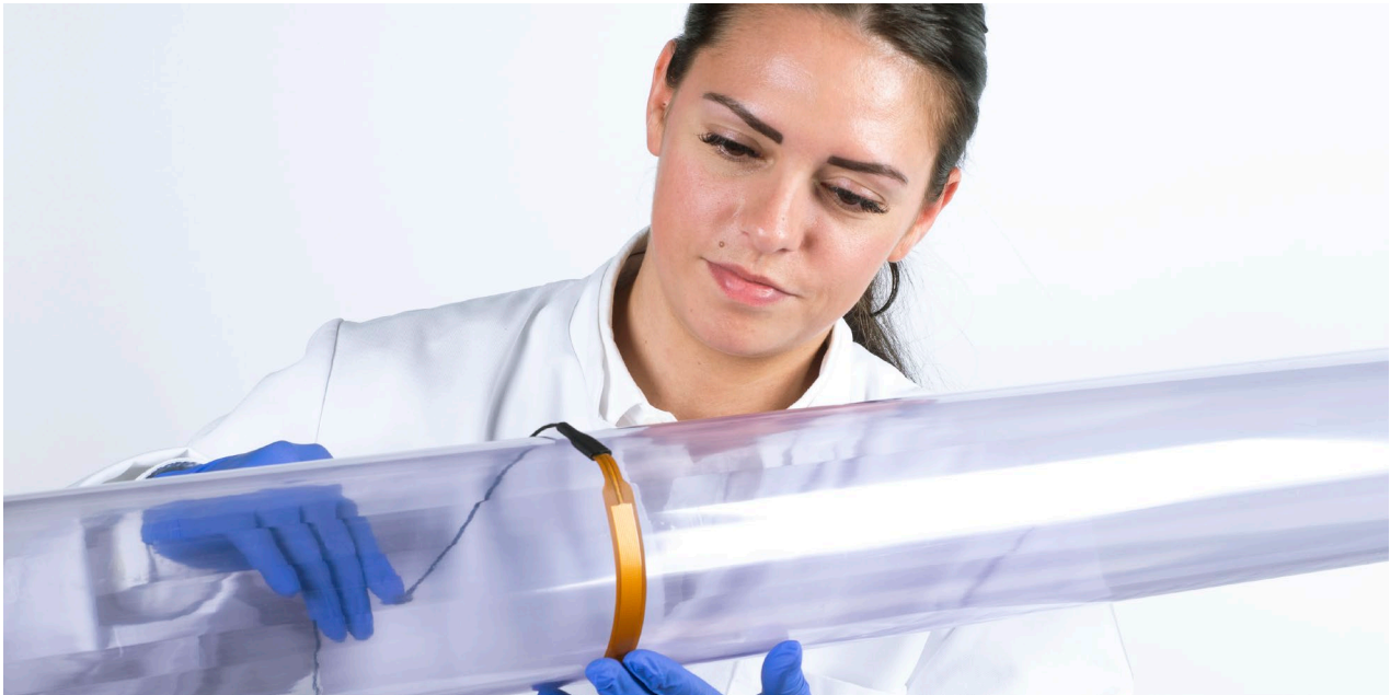
Figure 1 Flexible heat flux sensor FHF05-15X85 on a tube surface measuring heat flux between the tube and its environment.
