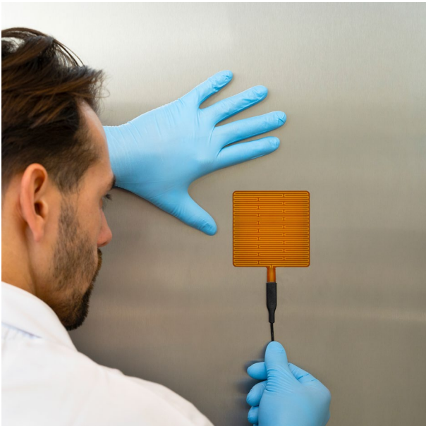
Figure 1 FHF05SC-50X50 Heat flux sensor mounted on a wall, using silicone glue (NR 5 in table 1). NOTE: sensor optical properties do not match those of the metal wall it will later be covered with a metal cover so that optical properties match (NR 4 in table 3).
