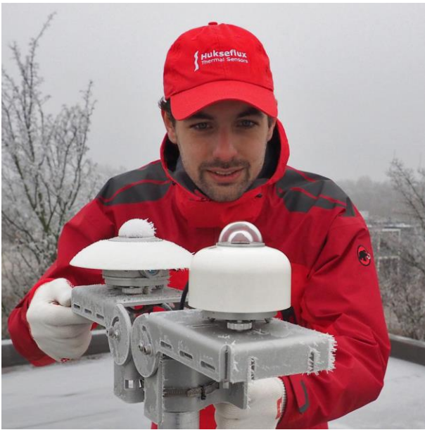
Figure 3 Hukseflux model SR30 (at the front) is the first heated pyranometer, compliant with the requirements of IEC 61724-1 for Class A monitoring systems. It overcomes a typical problem in freezing conditions seen with the non-heated pyranometer at the back: ice accumulation on the pyranometer dome surface reduces data availability.
