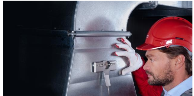
Figure 6 Mounting of IHF02 using an optional frame with magnets: note that optical properties of the sensor (black) do not match those of the metal object on which the sensor is mounted. This will lead to bad measurement data. (see also figure 3).
