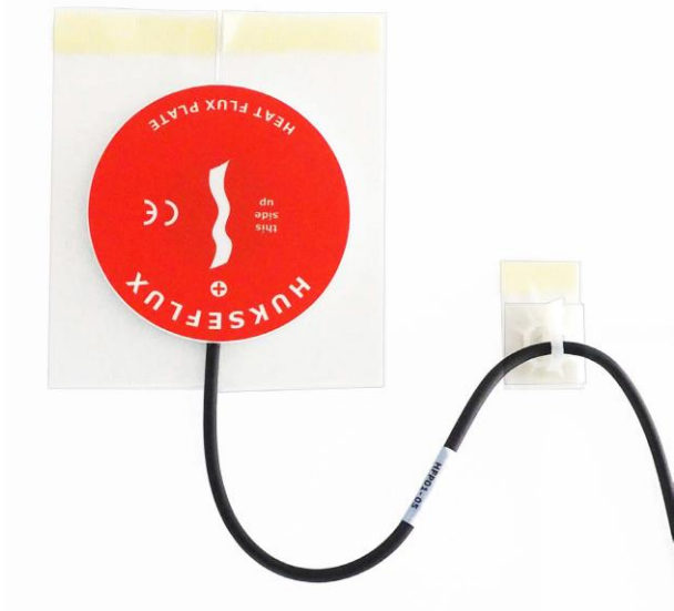
Figure 2 Installation of HFP01 on a wall using 2-sided "removable" carpet laying tape such as TESA 4939 (table 1, NR4) and a strain relief of the cable using a cable tie mount equipped with the same carpet laying tape as adhesive. Note that the optical properties in the visible range do not match those of the surrounding wall. This is acceptable if the heat transfer by visible radiation is negligible, in other words if there is no solar radiation or illumination by strong lamps.
