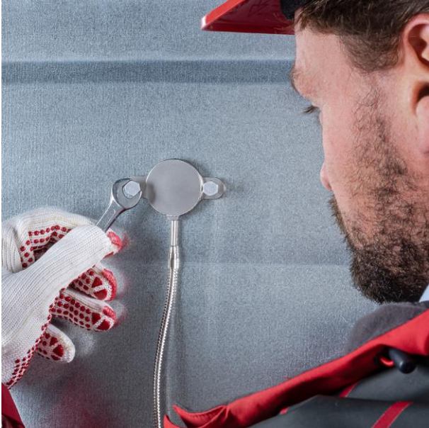
Figure 3 IHF02 industrial heat flux sensor bolted to the surface. Note that the optical properties of sensor and surrounding metal are matching (both blank metal). Springs are not visible.
