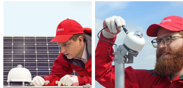
Figure 3 ventilation can be used to reduce thermal gradients and thereby zero offsets. Left: an SR20-D2 pyranometer mounted on a VU01 ventilation unit for external ventilation. Right: an SR30-D1 pyranometer with internal ventilation.
