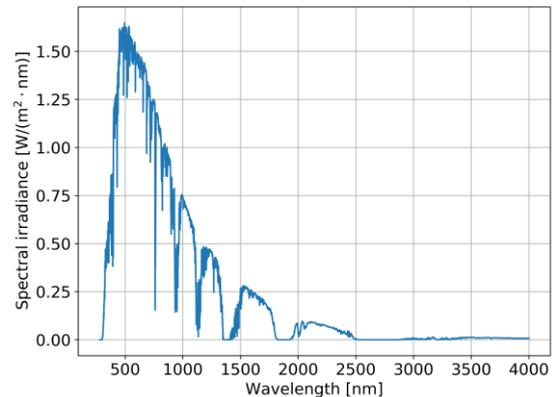
**Figure 3** The spectral distribution of a global tilted irradiance (GTI). Data from the ASTM G173-03 Reference Spectra.
