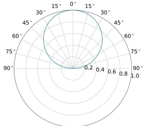
**Figure 5** A polar plot of the Lambertian or cosine directional response (distance to origin corresponds to  $E_{\text{gl}}/E = \cos(\theta)$ ) of a pyranometer as a function of the angle of incidence. The directional response is 1 for an angle of incidence of  $0^\circ$  and 0 for an angle of incidence of  $90^\circ$ . Pyranometers are not sensitive to light coming from the bottom.
