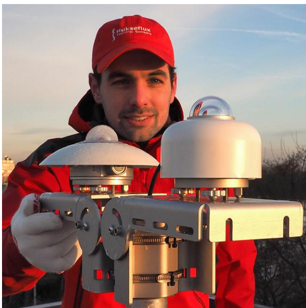
Figure 1 dew formation on a pyranometer (left) with a temperature below the dew point temperature
