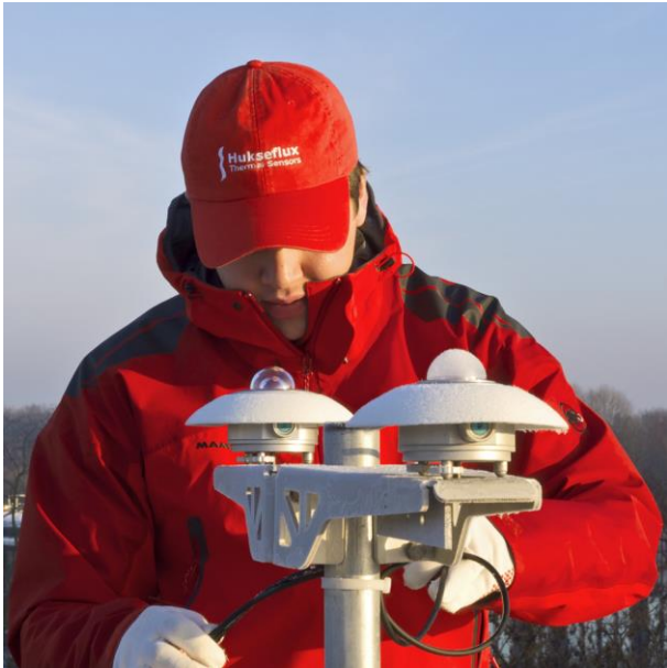
Figure 3 a SR25 (left) is heated just above frost point to prevent the formation of frost, while frost has formed on the dome of a SR20 (right) below frost point
