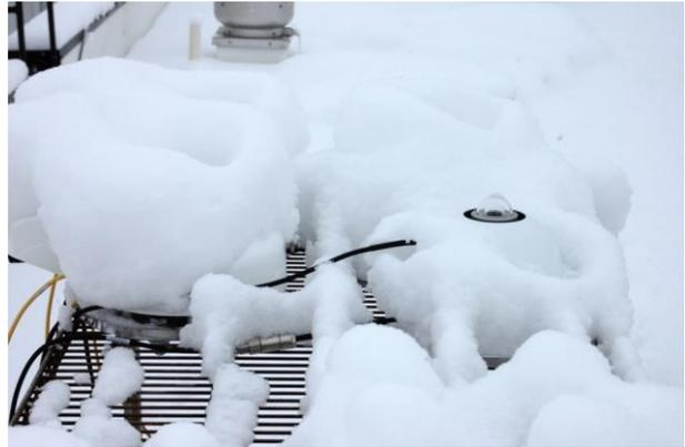
**Figure 5** Does ventilation work to remove snow? Not reliably: this photo shows 3 ventilation units in FEB 2014 in Logan UT, USA powder snow. Only 1 of the 3 pyranometers, the one at the right (SR20 with VU01), is visible. The other 2 are still covered in snow. Photo courtesy of Apogee Instruments Inc.
