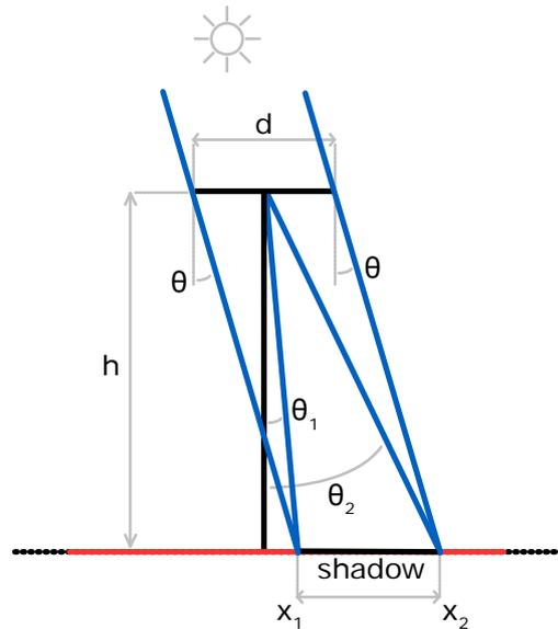
**Figure 5** schematic drawing of the shadow cast by an albedometer with a diameter  $d$  for a certain solar zenith angle  $\theta$
