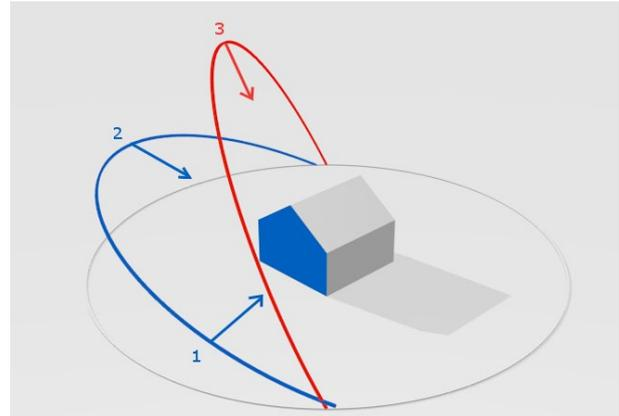
Figure 2 incidence angles change during day and season. During morning in winter (1), the indicated façade receives a lot of sun. In the afternoon this is greatly reduced (2). In summer, much more light is reflected and the roof will receive more sun (3).
