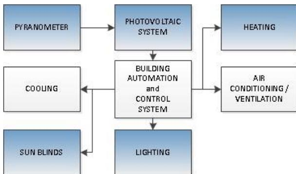
**Figure 3** BACS with integrated pyranometer
