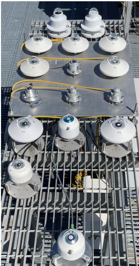
Figure 1 NREL's Global Horizontal West Table with among others Kipp & Zonen SMP12, EKO MS-80S, and Hukseflux SR30. Image credit: NREL SSRL BMS.
