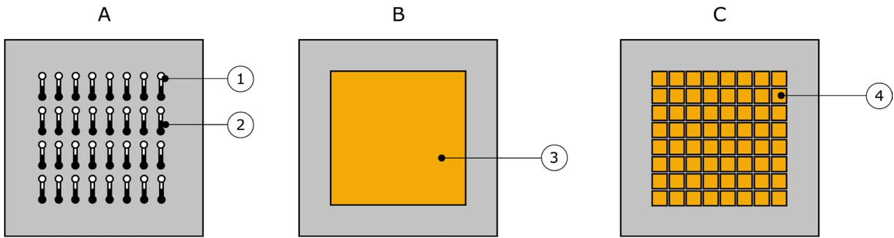
**Figure 3** A: sensor without a spreader such as Omega model HFS-5. One thermopile alloy (1), other thermopile alloy (2) In B and C, the thermopile is covered by spreaders. B: sensor with a single large spreader (3) C: sensor with multiple small spreaders (4) such as the FHF05-series sensors made by Hukseflux.
