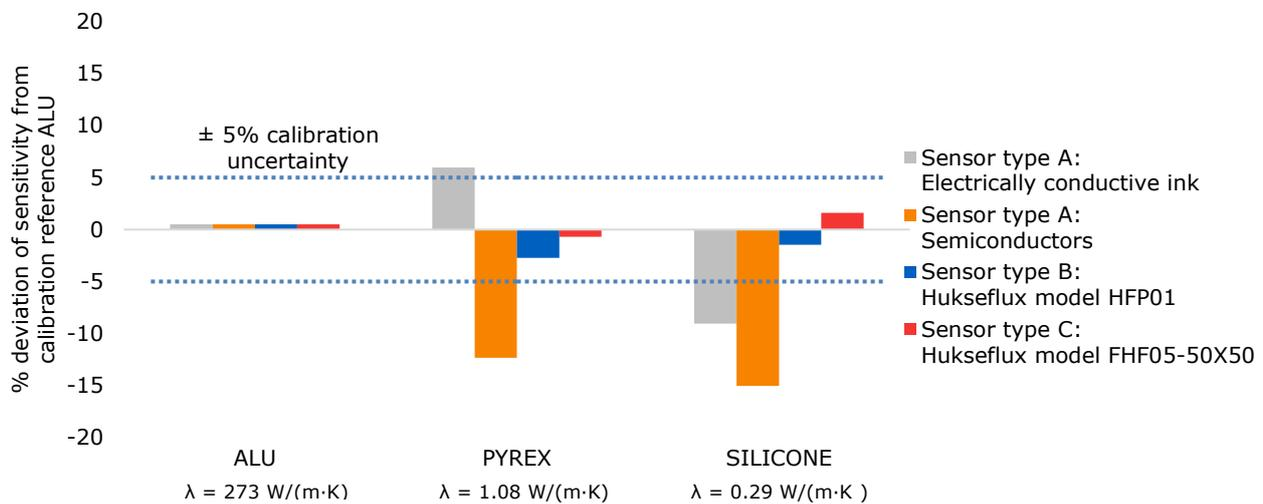
**Figure 4** Thermal conductivity dependence of three sensor types. Two "type A" sensors were tested: one Omega with a thermopile made of electrically conductive inks and the other made of semiconductors. The calibration uncertainty is 5%. The Omega HFS-5 makes up to 10% error when the thermal conductivity of the environment changes. Errors made with type B and C – Hukseflux FHF05-series sensors – are negligible.
