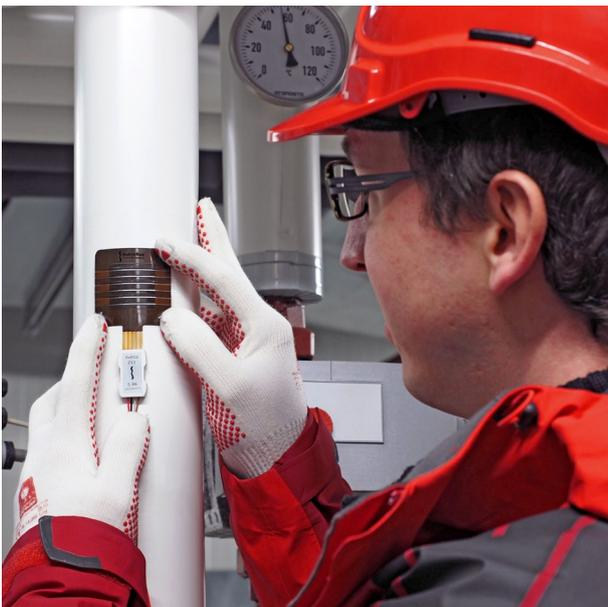
**Figure 2** FHF02 heat flux sensor installed on a pipe
