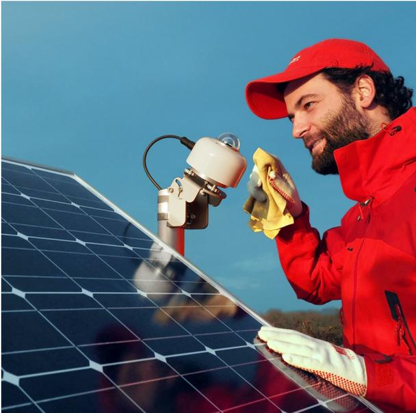
**Figure 1** SR30 pyranometer for PV system monitoring
