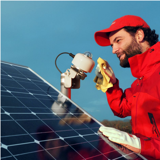
Figure 1 SR30 pyranometer for PV system monitoring
