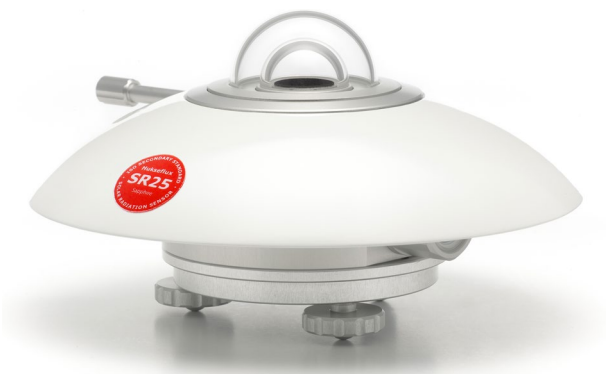
Figure 2 Example of a Hukseflux pyranometer: SR25 secondary standard pyranometer with sapphire outer dome. This model is recommended for research grade diffuse radiation measurement. Output is either analogue millivolt or digital via Modbus RTU over RS-485 and analogue 4-20 mA (current loop).
