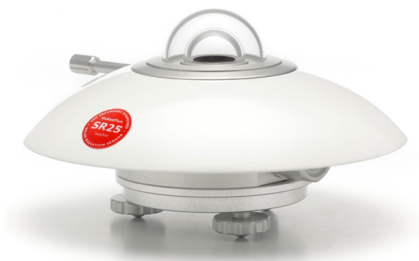
Figure 2 Example of a Hukseflux spectrally flat Class A pyranometer, model SR25, with a sapphire outer dome. This model is recommended for research grade diffuse radiation measurement. Output is either analogue millivolt or digital via Modbus RTU over RS-485 and analogue 4-20 mA (current loop).
