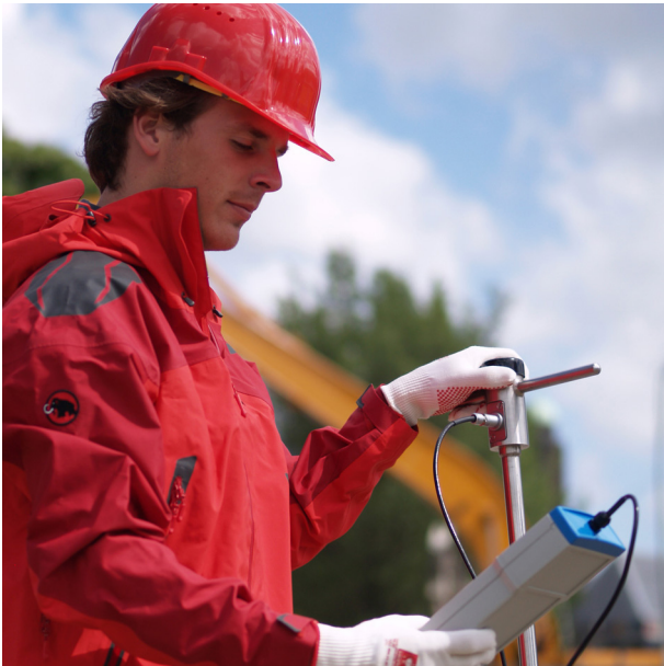
Figure 1 Example of an application of Hukseflux thermal conductivity measuring systems: thermal route survey
