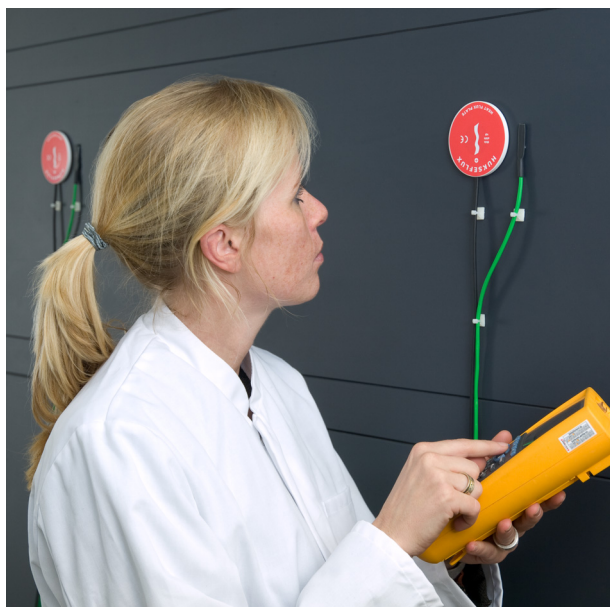
Figure 4 TRSYS01 system in use for building envelope thermal resistance measurement
