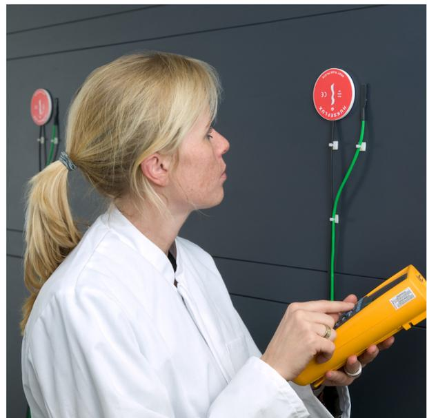
**Figure 3** HFP01 in use: on-site measurement of the building envelope thermal resistance
