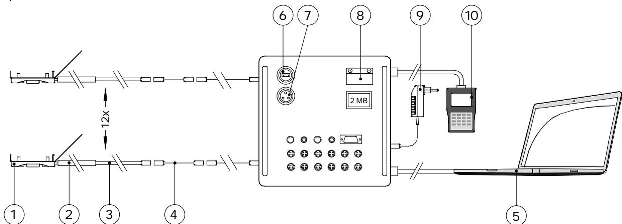
**Figure 2** the ALUSYS measuring system; (1) HF01 heat flux sensor (with magnet frame), (4) low temperature extension cables with 2 connectors, (5) PC or laptop (not part of the system). On or inside the MCU: (6) chassis connector for PC connection via USB,
