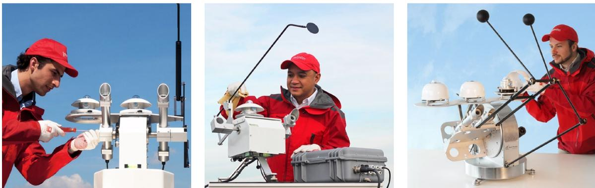
**Figure 0.3** Applications of DR01, DR02 and DR03 pyrheliometers, combined with SR20 pyranometers, in typical solar radiation monitoring stations
