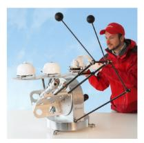
**Figure 0.3** Applications of DR01, DR02 and DR03 pyrheliometers, combined with SR20 pyranometers, in typical solar radiation monitoring stations
