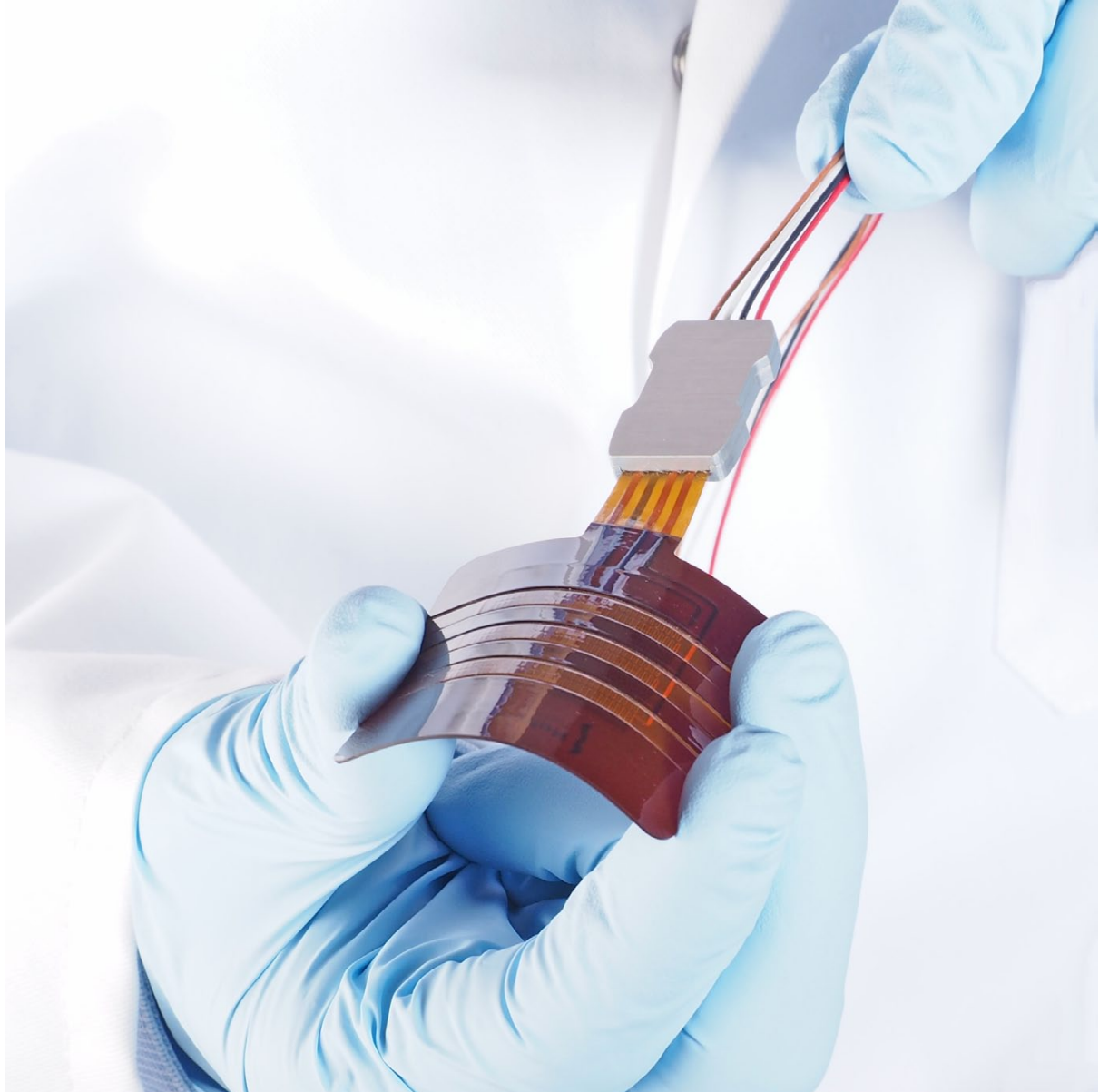
Figure 5.2.1 Bending direction of a foil heat flux sensor similar to FHF02. Bending the FHF02 in this direction minimizes the strain on the sensor and improves the measurement result
