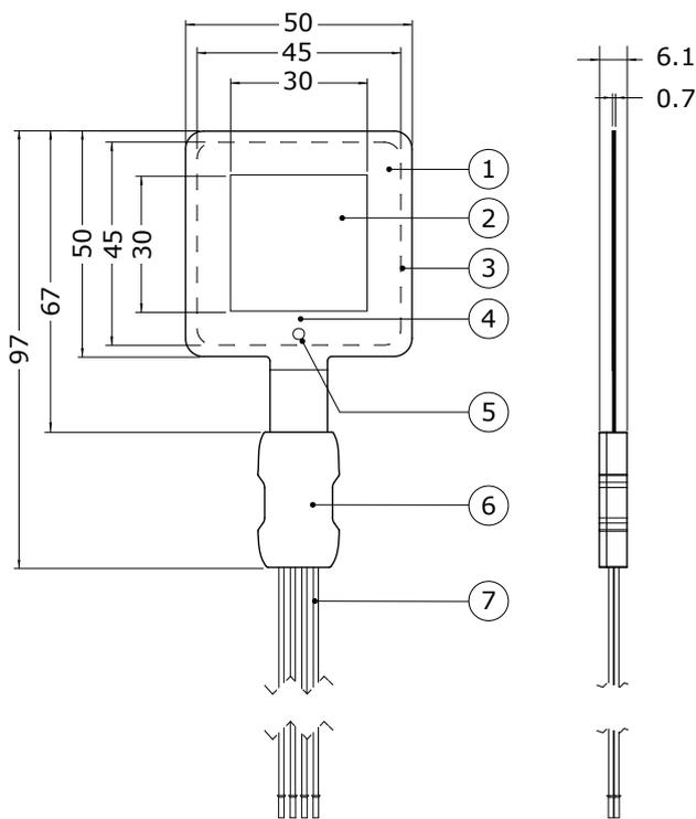
**Figure 4** FHF04SC heat flux sensor: (1) sensing area with thermal spreaders, (2) passive guard, (3) contour of the heater area for self-test, (4) type T thermocouple, (5) dot indicating front side, (6) metal connection block showing serial number and sensitivity, (7) wires, standard length is 2 m. Dimensions in  $\times 10^{-3}$  m.
