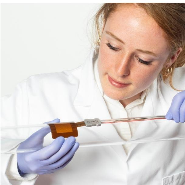
**Figure 2** FHF04SC being installed to measure heat flux on a curved surface
