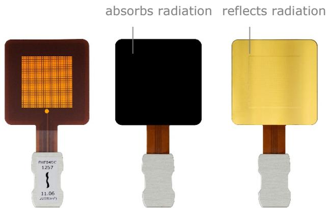
**Figure 6** FHF04SC heat flux sensor: with BLK-5050 and GLD-5050 stickers
