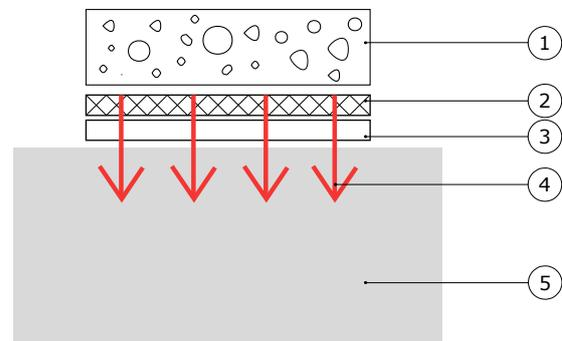
**Figure 3** Calibration of FHF04SC; a typical stack used for calibration consists of a block of metal (mass > 1 kg), for example aluminium (5), the heat flux sensor (3), with heater (2) and an insulation foam (1). Under these conditions, heat losses through the insulation are negligible. Heat flux (4) flows from hot to cold.
